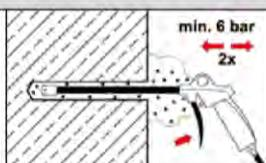
Starting from the bottom or back of the bore hole, blow the hole clean with compressed air (min. 6 bar) a minimum of **two** times. If the bore hole ground is not reached an extension shall be used.
