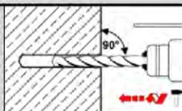
Drill a hole into the base material to the size and embedment depth required by the selected anchor (Annex B2). In case of aborted drill hole: the drill hole shall be filled with mortar.
