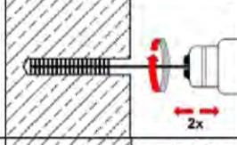
Attach the brush to a drilling machine or a battery screwdriver. Brush the hole with an appropriate sized wire brush  $> d_{b,min}$  (Table B4) a minimum of **two** times. If the bore hole ground is not reached, a brush extension shall be used.
