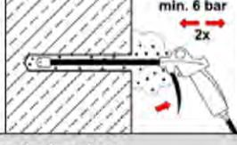
Finally blow the hole clean again with compressed air (min. 6 bar) a minimum of **two** times. If the bore hole ground is not reached an extension shall be used.
