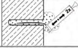
Finally blow the hole clean again with the blow-out pump a minimum of **two** times. If the bore hole ground is not reached an extension shall be used.
