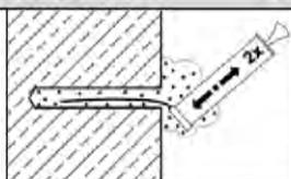
Starting from the bottom or back of the bore hole, blow the hole clean with the blow-out pump minimum of **two** times. If the bore hole ground is not reached an extension shall be used.
