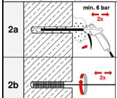
Starting from the bottom or back of the bore hole, blow out the hole with compressed air (min. 6 bar) a minimum of **two** times until return air stream is free of noticeable dust.
