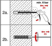
Starting from the bottom or back of the bore hole, blow out the hole with compressed air (min. 6 bar) a minimum of **two** times until return air stream is free of noticeable dust. If the bore hole ground is not reached, an extension must be used.
