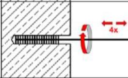
Check brush diameter (Table B4). Brush the hole with an appropriate sized wire brush  $\geq d_{b,min}$  (Table B4) a minimum of **four** times.
