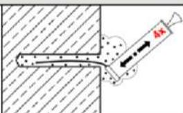
Starting from the bottom or back of the bore hole, blow out the hole with the blow-out pump a minimum of **four** times.
