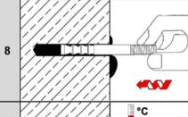
Insert the anchor rod VMZ-A by hand, rotating slightly up to the full embedment depth as marked on the anchor rod. The anchor rod is properly set when excess mortar seeps from the hole (Pre-setting installation) or the annular gap in the clearance hole in the fixture is completely filled by excess mortar (Through-setting installation). If the hole is not completely filled, pull out anchor rod, let mortar cure, drill out hole and repeat entire cleaning process.
