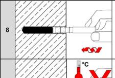
Insert the anchor rod VMZ-IG by hand, rotating slightly up to about 1 mm below the concrete surface in the drill hole. The anchor rod is properly set when excess mortar seeps from the hole. If the hole is not completely filled, pull out anchor rod, let mortar cure, drill out hole and repeat the entire cleaning process.
