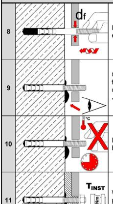
Insert the anchor rod VMZ-A by hand, rotating slightly up to the full embedment depth.
