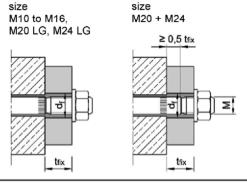
The annular gap in the clearance hole in the fixture has to be filled completely by excess mortar!
