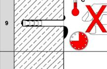
Follow minimum curing time shown in Table B1 and Table B2. During curing time anchor rod must not be moved or loaded.
